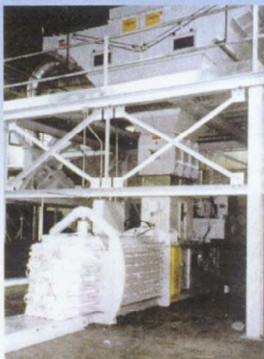
AIRSCREEN system feeding an auto-tie baler.
