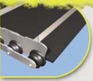
**Combination Belt Conveyors** are heavy-duty conveyors that feature a chain drive system incorporated with a rubber belt for medium to high volume applications ranging from 5 to 30 tons/hour.
